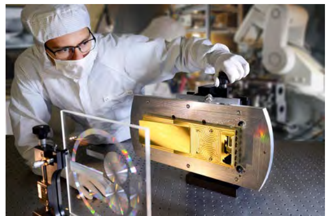
Metrology of a mirror module having two freeform surfaces and reference structures with a computer generated hologram.
